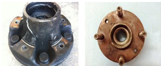
Fig 1. Crack near the hub
